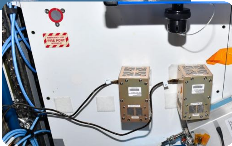
Two photocatalytic air purifiers installed on board the International Space Station (ISS) (Credit: NASA/Axiom)
